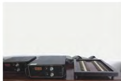
Integrator Machine Set (To test Color Temperature, Luminous Flux, Ra ...)
