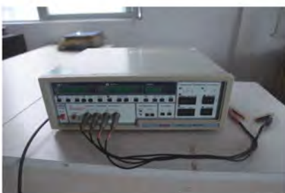
LCR Test Machine (To test Electrical resistance, Capacitance, Inductance)
