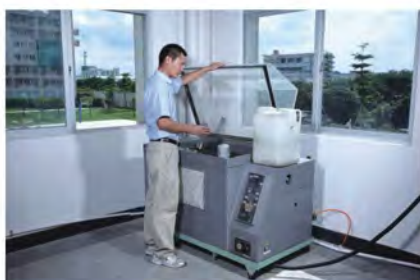
Salt Spary Test Machine (To test Anti-corrosion status of metal material)
