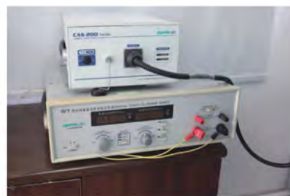
LED Luminous Intensity Meter (To test the bright of LED)
