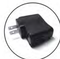
AC-USB Adaptor I/P 100-240V AC 50/60Hz O/P 5V DC 500mA
