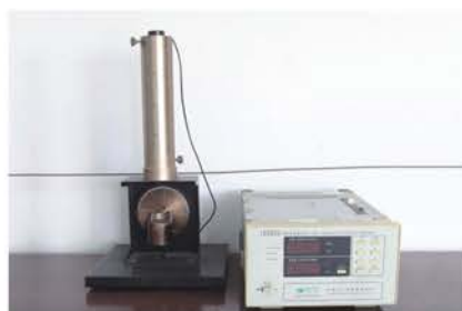
LED Aging Test Machine (Mainly use to test High Power LED)
