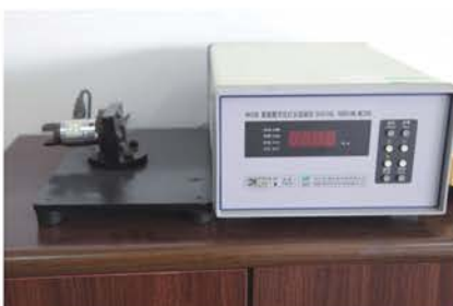
Lampholder Torsion Test Machine (Torsion test after the lampholder is assembled)
