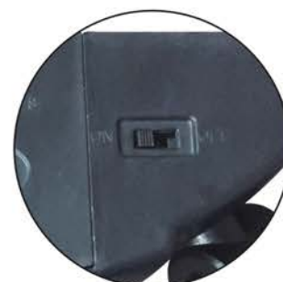
Slide Switch: ON(Auto)/OFF
