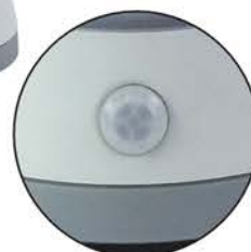
PIR + CDS Sensor Version CDS: Working when < 10Lux PIR: 2.5M, 20S, Horizontal 100°, Vertical 50°
