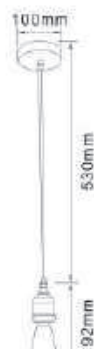
● HG-947 Material: Aluminum + PVC Wire Bulb Adaptable: E27 6W LED Bulb Finish: Antique Brass / Copper
