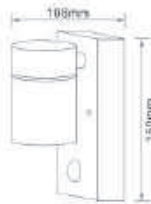
● EL-426DNS GU10 5W LED Bulb With Sensor Sensor Range: 8M x 120°
